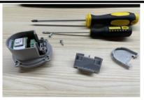
3. Remove the cover and unscrew the LED board
