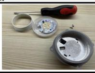
2. Unscrew and remove the metal shell
