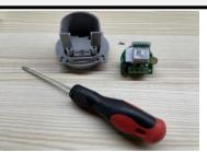
4. Unscrew and remove the fixing plate and pry open the back cover
