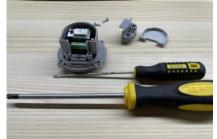
3. Remove the cover and unscrew the LED board
